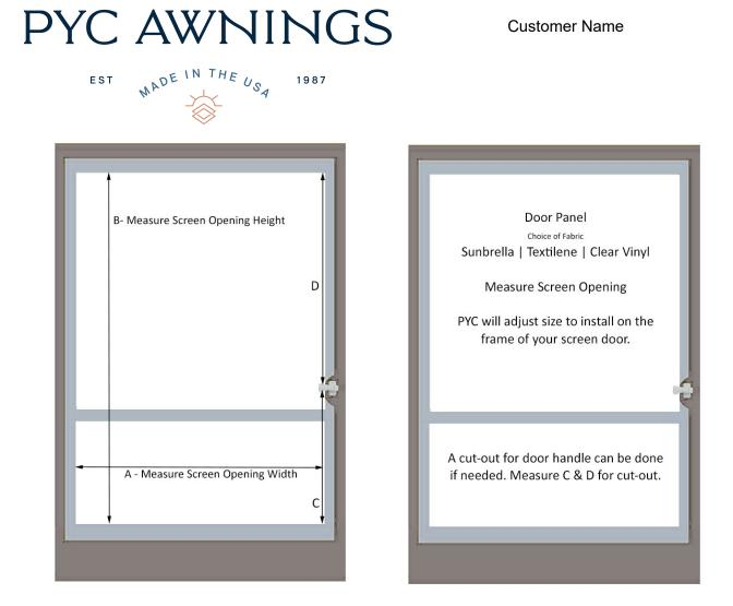
When measuring, measure on the side of the door you where you will install the panel.
