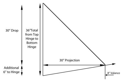
Measure the width where hinges of awning will be mounted. All awning hardware shoud be mounted on either window frame or exterior wall to keep the awning level.
